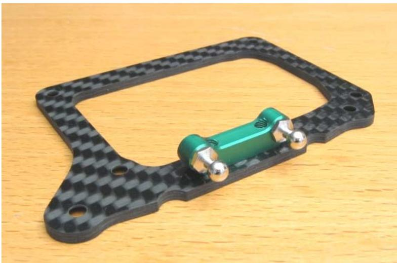
Further two ball screws M3 are to be mounted on the pivot block with Loctite medium. Then fix the unit with two countersunk screws M3x6 onto the Power pod bottom plate.
