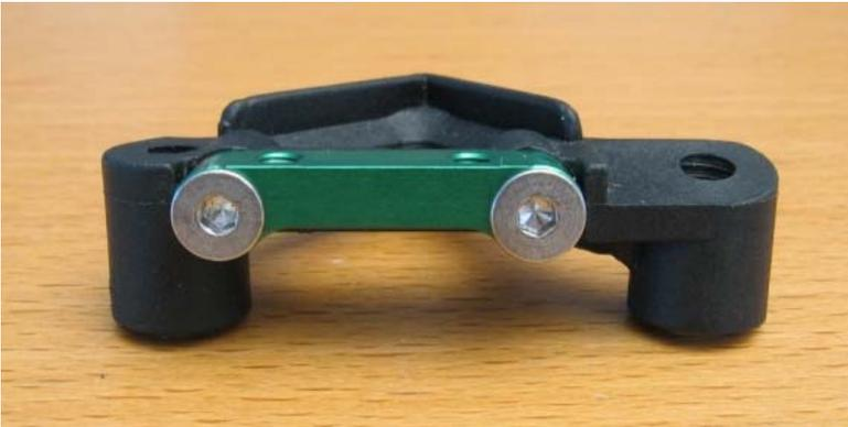
The two front axle blocks are fixed with countersunk screws M3x10 to the original Asso / Calandra / IRS front axle supports.
