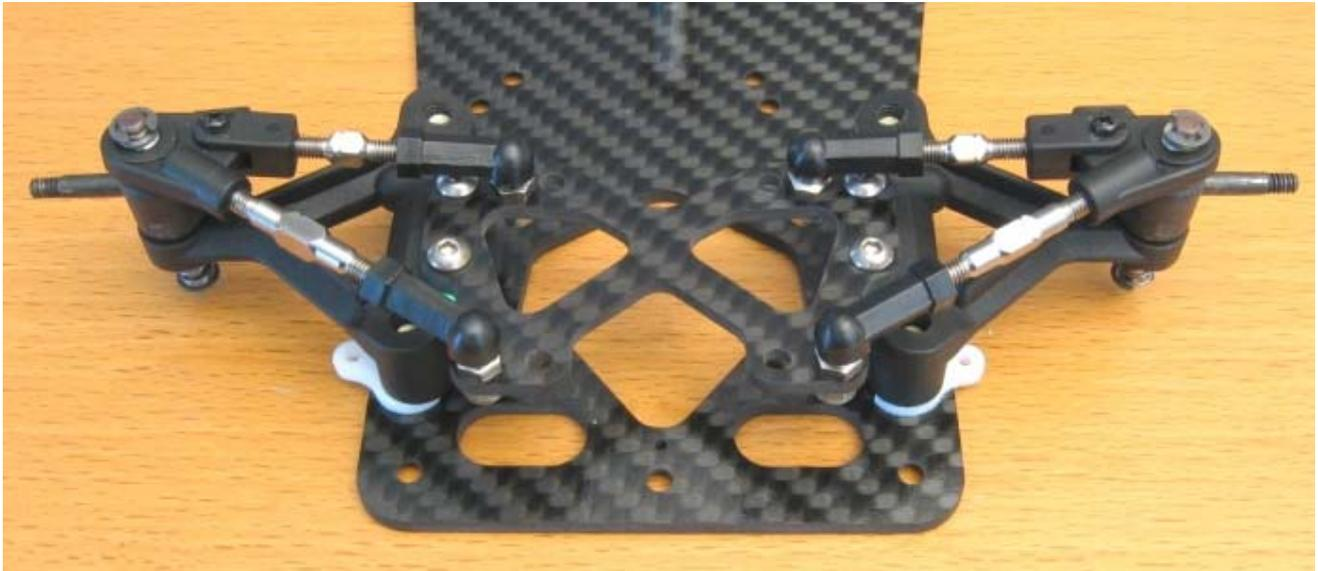
The front axle will now be completed with the upper links of the Cross conversion kit. The extreme low clearance GM links should be used as internal joint heads. The ball joints of the Cross kit are well suited as steering link joints as they are very smooth-running.
