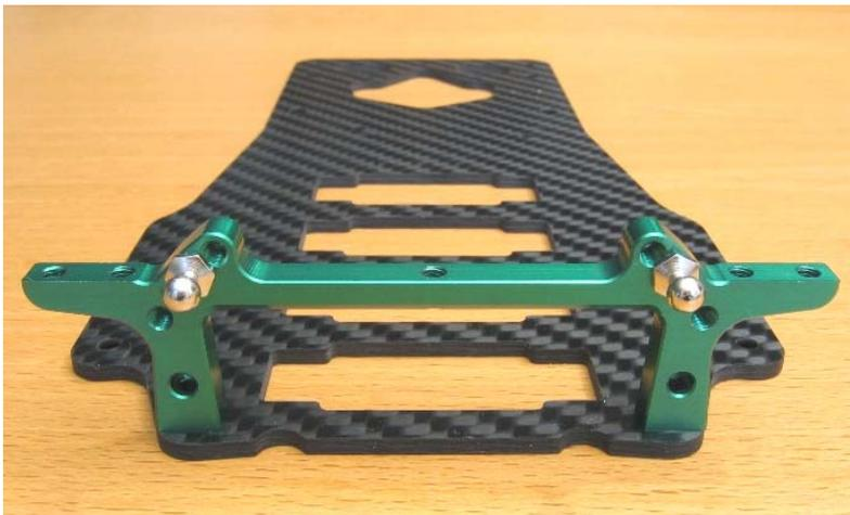
Mount ball screws with Loctite medium at bridge position 3 (second from top) and fix the unit with two countersunk screws M3x6 on the chassis.
