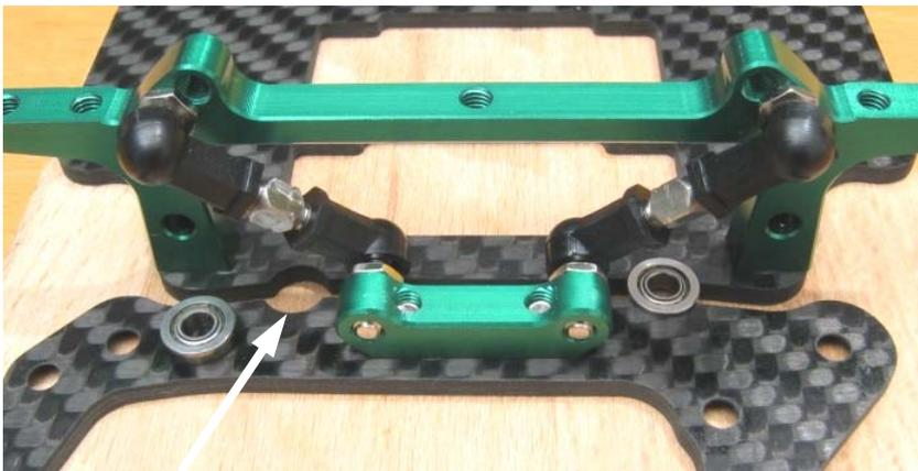
The chassis and the power pod bottom plate have opposing semicircular clippings each. Insert an adjustment disc of 6mm diameter into each clipping for correct adjustment (such as a ball bearing 3x6mm).
