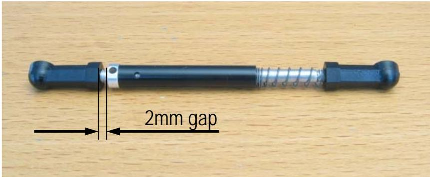
Preassemble Corally tubes with long GM ball buttons (in contrast to the original parts they have no clearance, the damping works more directly).
