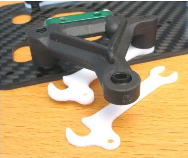
Mount those blocks with aluminum screws to chassis. To compensate the tire diameter there are spacers available in 0,5mm, 1mm and 2mm. Plug in the spacers at the rear attachment point and pivot them below the front attachment point. For the exchange of the spacers you need not turn out the screws completely.
