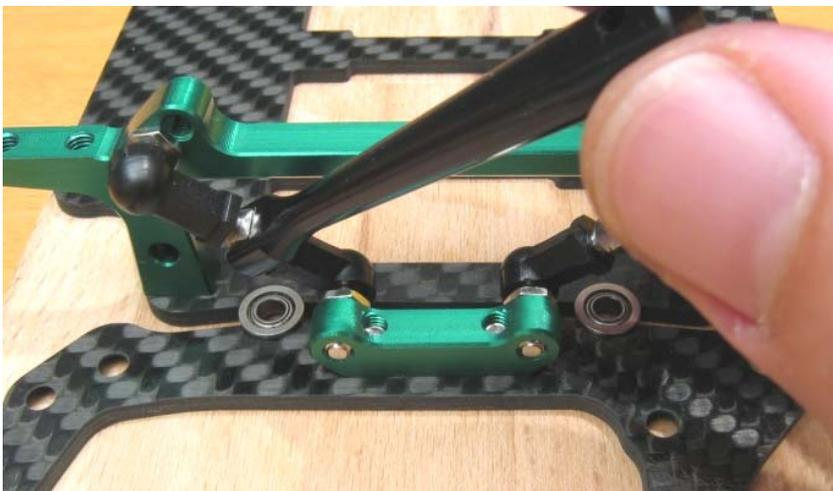
The V-links are adjusted correctly if both discs are fitting flush into the cut-outs and the chassis as well as the power pod are even on a plane surface.
